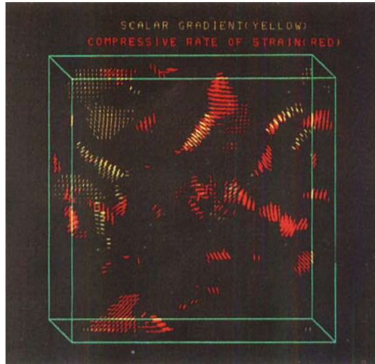
FIGURE 18. Three-dimensional perspective plots of the compressive component of the rate-of-strain (red) and scalar-gradient (yellow) fields. 1000 lines are plotted for the rate of strain. 500 lines are plotted for the scalar gradient. The perspective is the same as in figures 13(a) and 14(a). The rate-of-strain structure in the top centre is aligned along the scalar-gradient structure with the compressive component of the rate of strain parallel to the scalar gradient.
