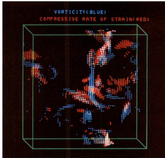
FIGURE 16. Three-dimensional perspective plots of the vorticity (blue) and compressive component of the rate-of-strain (red) fields. Short lines in the direction of the compressive component are plotted at the points of a 64^3 mesh if the total rate of strain is above a threshold. 1000 lines are plotted for the rate of strain. 2000 lines are plotted for the vorticity. (a) The same perspective as in figures 13 (a) and 14 (a). The rate-of-strain structure in the top centre is aligned along the vortex structure with the compressive component of the rate of strain perpendicular to the vorticity. (b) The same field as (a), but rotated 90^\circ about the vertical axis. It has the same perspective as figure 14 (b). The rate-of-strain in (a) which is aligned with the vorticity is the fanlike structure in the upper centre.
